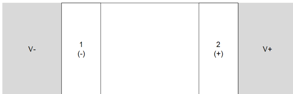
Figure 26. Recommended Layout: DEC Package
