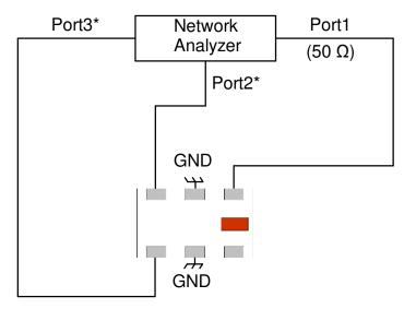
\*Impedance for ports 2 and 3=1/2(Balanced impedance)
