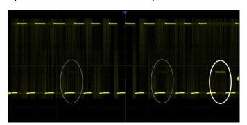
With a waveform update rate of up to 110,000 wfm/s, the oscilloscope can easily capture unusual or low-probability events. In Sequence mode the waveform capture rate can reach 500,000 wfm/s
