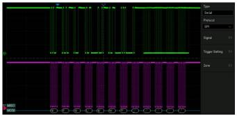
Display the decoded characters through the events list. Bus protocol information can be quickly and intuitively displayed in tabular form. I<sup>2</sup>C, SPI, UART, CAN, LIN, CAN FD, FlexRay, I<sup>2</sup>S, MIL-STD-1553B, SENT and Manchester are supported
