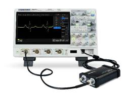
SDS5000X can control the SAG1021I USB Function/Arbitrary waveform generator to output waveform with up to 25 MHz frequency and ±3 V amplitude. Six basic waveforms plus multiple types of arbitrary waveforms are built-
