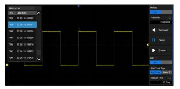
History function can record up to 100,000 frames of waveforms. The recording is executed automatically, so that the customer can play back the history waveforms at any time in order to observe unusual events and quickly locate the area of interest using the cursors or measurements. The failed frames of Mask Test can be stored as history
