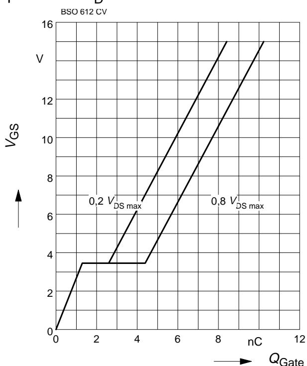
**Typ. gate charge (P-Ch.)** $V_{GS} = f(Q_{Gate})$ parameter:  $I_D = -2 \text{ A}$
