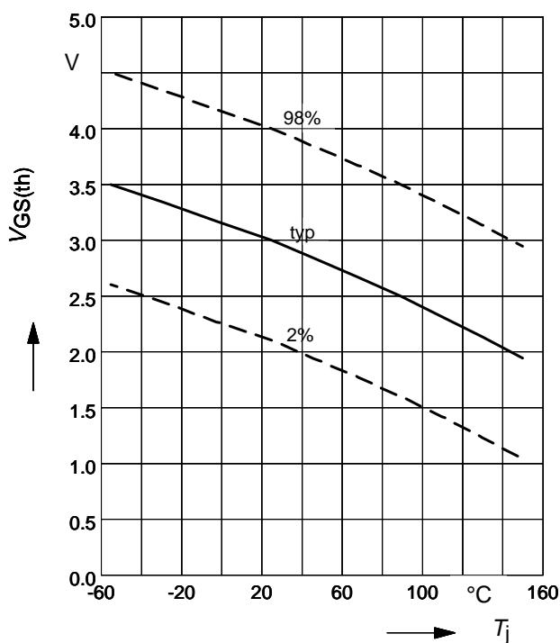
**Gate threshold voltage (P-Ch.)**
