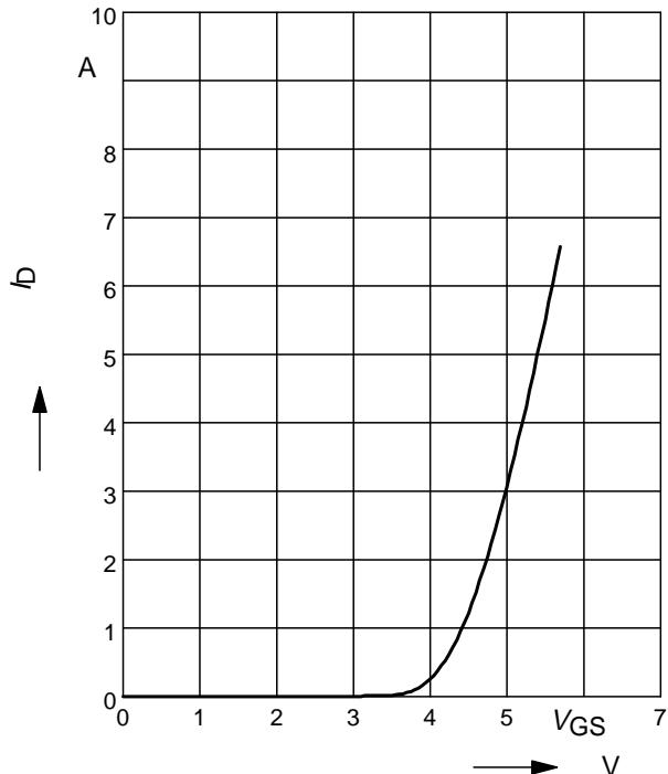
**Typ. transfer characteristics (P-Ch.)**parameter:  $t_p = 80 \mu\text{s}$
