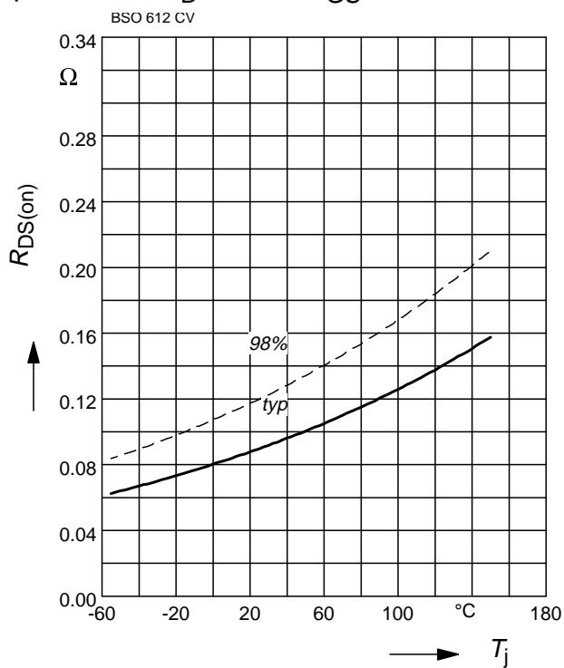
**Drain-source on-resistance (P-Ch.)**
