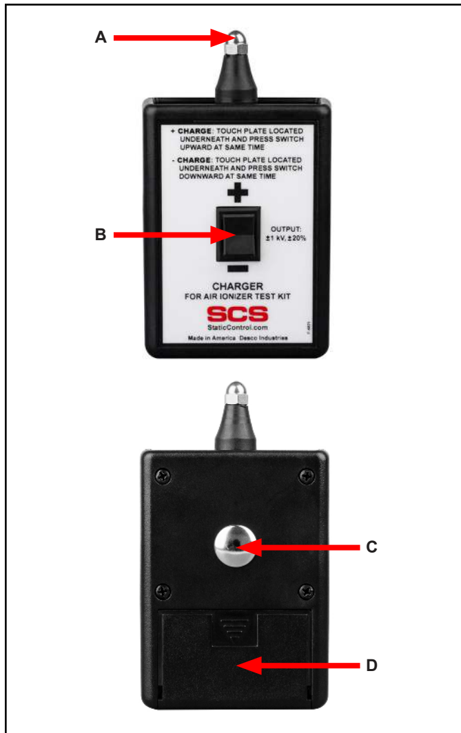
Figure 2. Charger features and components
