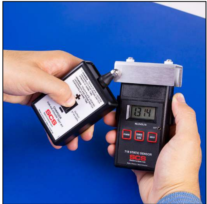
Figure 7. Charging the Conductive Plate on the Static Sensor
