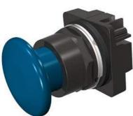
30mm BlackMax, Epoxy Coated Corrosion Resistant Metal Operator, Round Push-Pull Operator Non-Illuminated Mushroom Head Cap Small 1 3/4" (44.5 mm) Plastic, Blue 3 Position Pull-Momentary/Push-Maintained UL Listed, CSA Certified NEMA 1,3,3R,4,4X,12,13 & Automotive Standards
