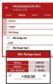
It automatically goes to the DATA tab, where we will see the parameters and we can modify them, accessing the drop-down menus (no longer having the mobile near the equipment).
