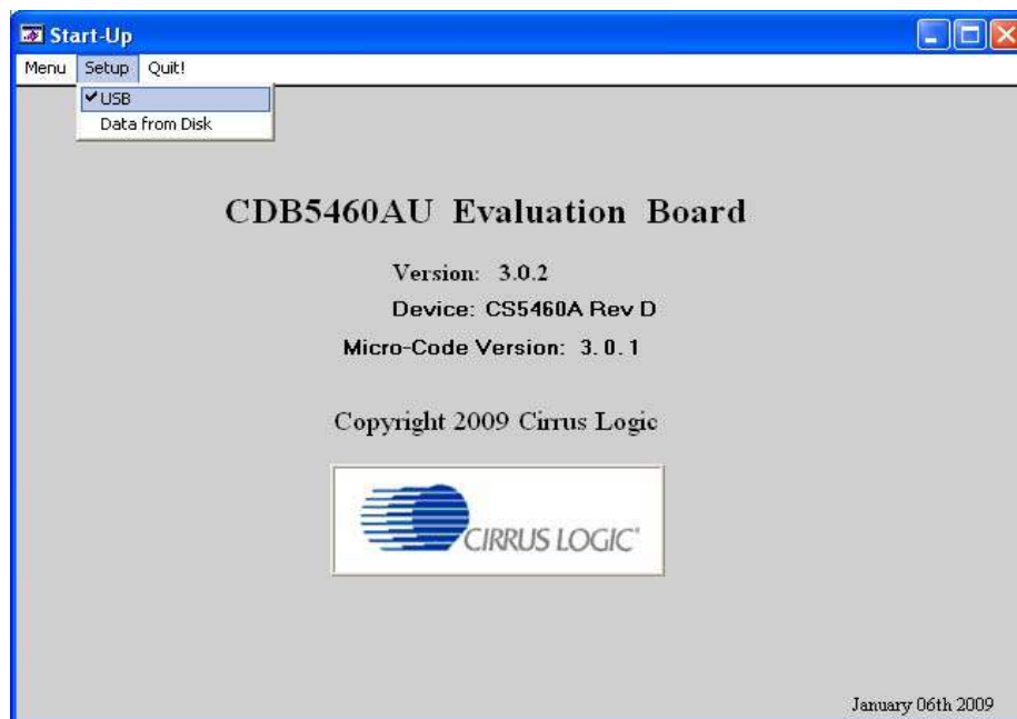
Figure 3. Setup Menu Showing Successful USB Connection
