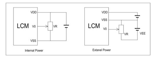
VDD-V0: LCD Driving Voltage
