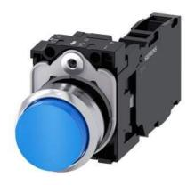
Pushbutton, 22 mm, round, metal, shiny, blue, pushbutton, raised, momentary contact type, with holder, 1 NO+1 NC, screw terminal
