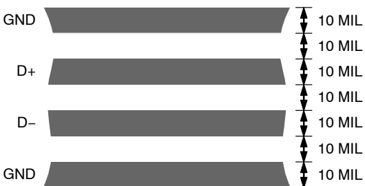
Figure 22. Arrangement of Signal Tracks
