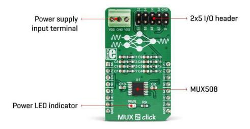
The MUX508 IC is targeted towards working with both bipolar and unipolar single-ended inputs. Each input is labeled as S1 to S8. When a specific channel is selected by using the A0 to A2 pins, it will be switched to the output pin, labeled as D. For the improved stability, each pin is equipped with the 100nF parallel capacitor and  $100\Omega$  series resistance. The input and the output signal pins are routed to the standard 2.54mm pitch 2x5 pins header on the Click board<sup>TM</sup>.
