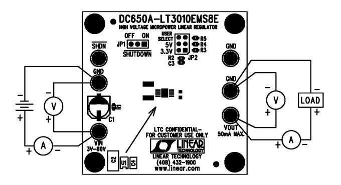
Figure 1. Proper Measurement Equipment Setup
