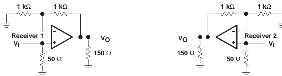
Figure 2. Receiver Input-to-Output Crosstalk Test Circuit
