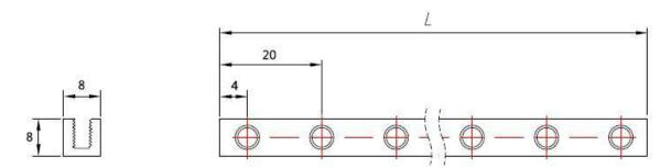
Note : In the middle of the thread groove is M4.
