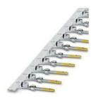
Crimp contact, Pin, rolled, Taped articles, number of pieces per reel: 500, contact diameter: 1 mm, crimp range:  $0.22~\text{mm}^2$  ...  $0.56~\text{mm}^2$ , Item is lead-free in accordance with RoHS II without Exemption 6c (Pb <0.1%)
