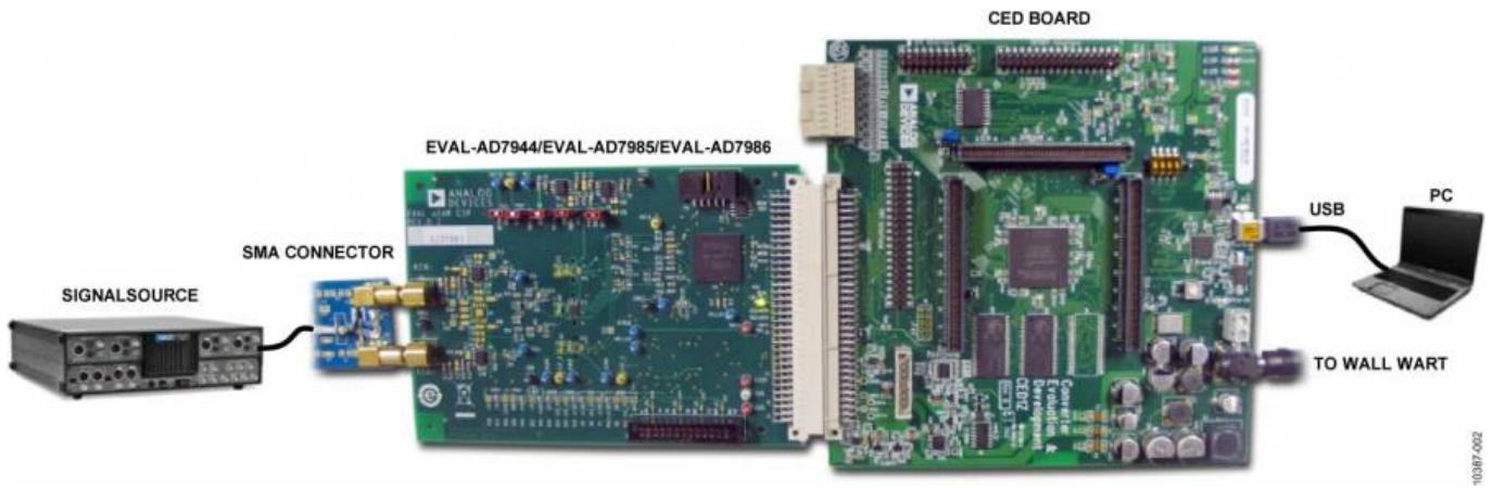
Figure 2. Hardware Configuration—Setting up the Evaluation Board
