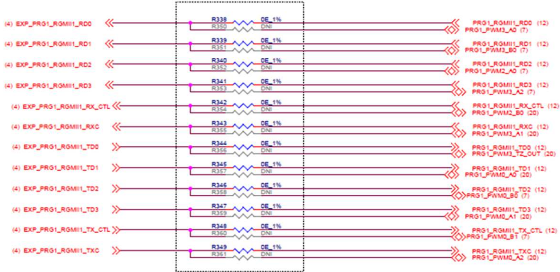
Figure 4-10. Resistor MUX for EXP_PRG1_RGMII1 Signal
