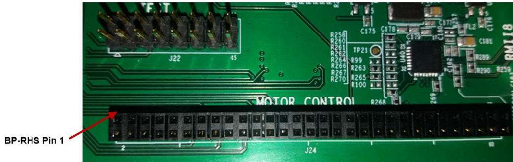
Figure 4-17. Motor Control Header
