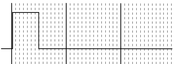
DS-1 (50% duty cycle) Arbitrary Waveform Example
