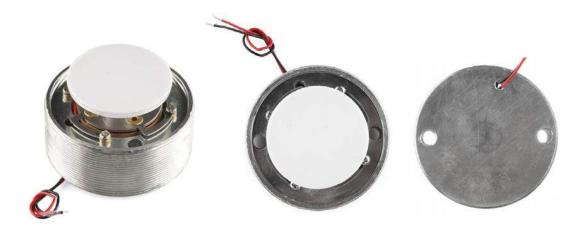
**Description:** Surface transducers give you the awesome power to turn almost any surface into a speaker. They're essentially just a speaker except instead of a cone, the coil is attached to a pad that conducts the vibration into whatever you press it against. Hook it up to an audio source and press it against the nearest table, wall or cardboard box. You can even put it against your head and play music directly into your skull (the ultimate surround sound).
