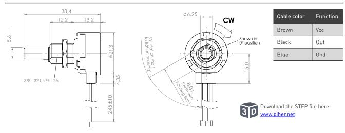
Sensor shipped with one nut installed at base. Assembled washer and extra nut available on request. Other shafts available on request.
