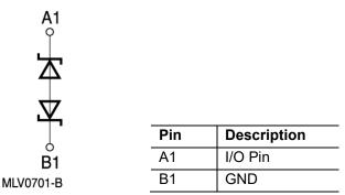
Due to the symmetrical configuration no marking information is needed.
