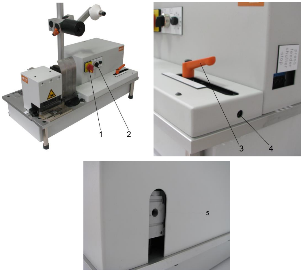
Fig. 22: Adjusting the feeder cylinder
