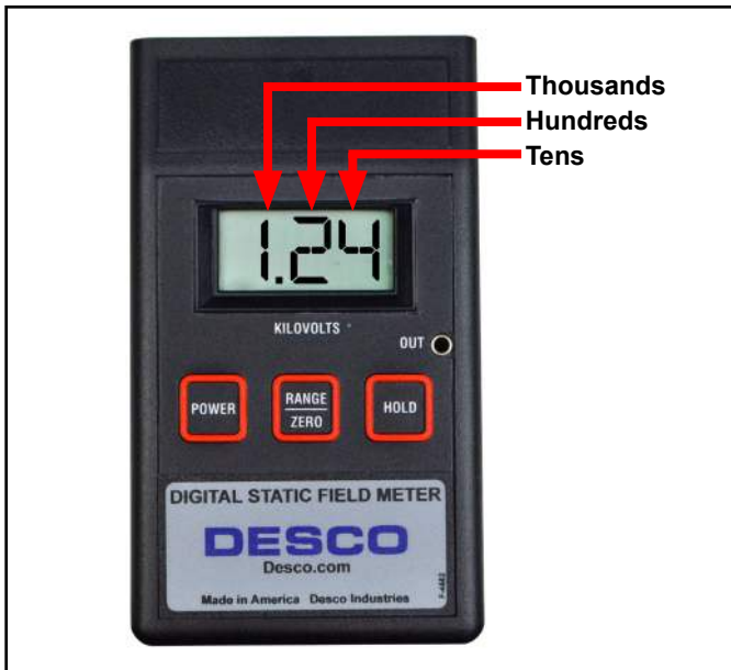
Figure 3. Reading the Digital Static Field Meter while in the \pm 20 kV range
