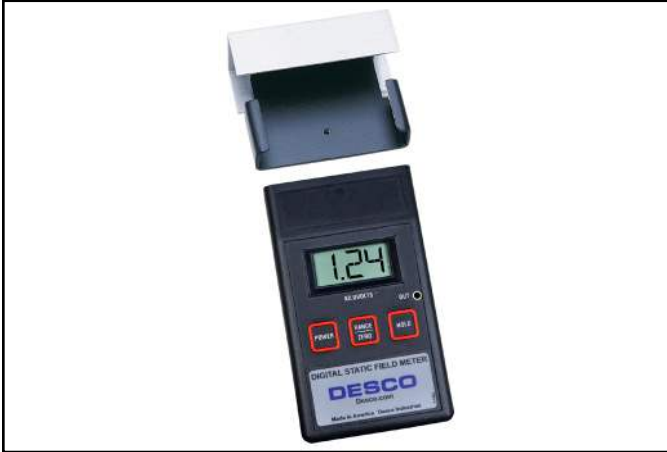
Figure 5. Installing the 19441 Conductive Plate
