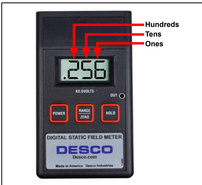
Figure 4. Reading the Digital Static Field Meter while in the \pm 2 kV range
