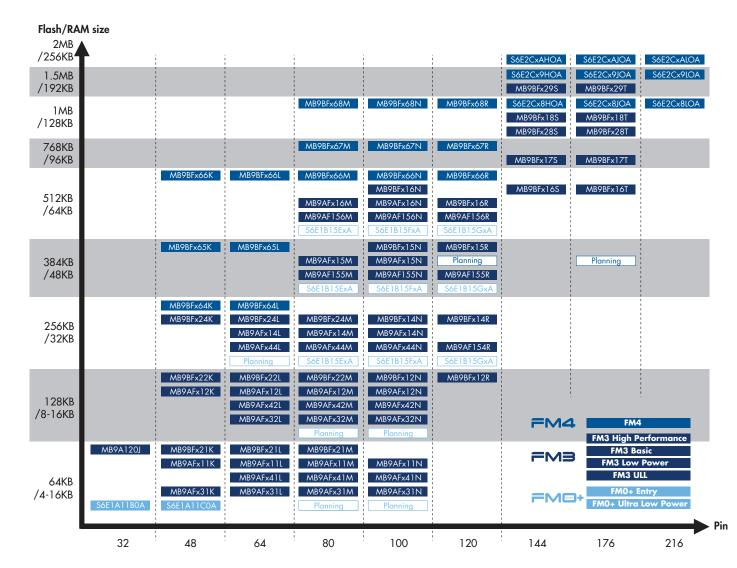
The Cypress FM MCU lineup consists of three families—FMO+, FM3 and FM4—each of which uses a specific ARM Cortex-M core. Users can easily transition between device types and families because of the compatibility of the instruction sets.
