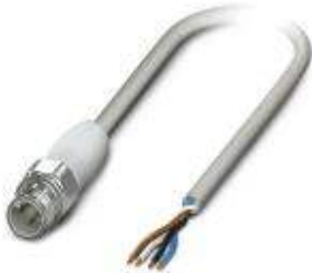
Sensor/Actuator cable, 4-position, PP-EPDM halogen-free, Gray RAL 7035, Plug straight M12, A-coded, on Free cable end, Cable length: 10 m, Hygienic design, With high-grade steel knurl
