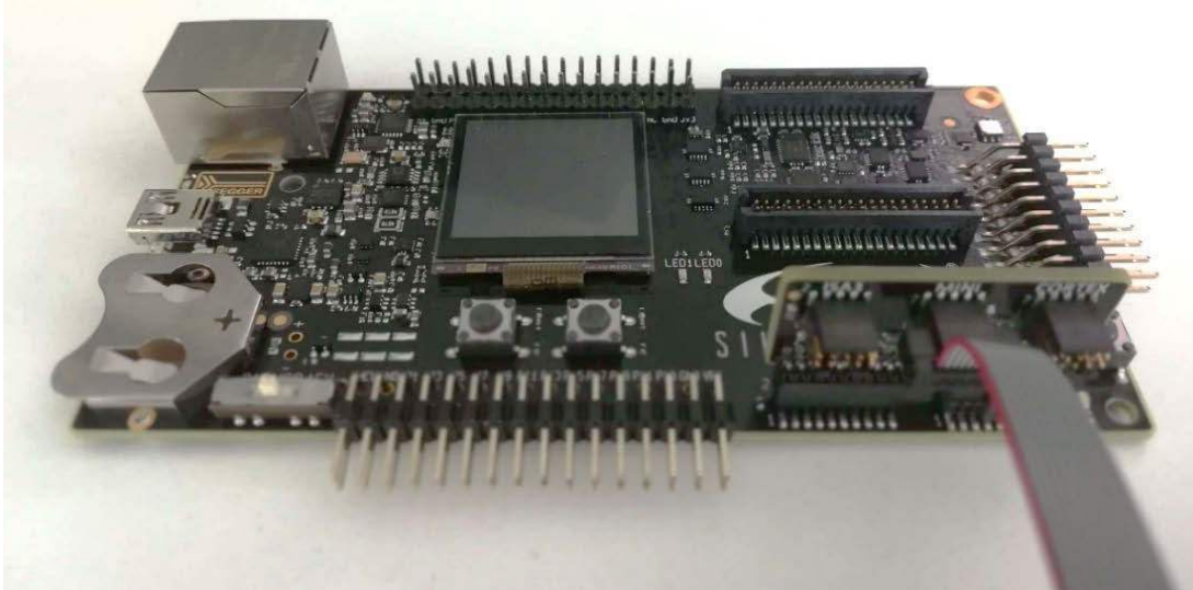
Figure 4.2 WSTK Board with STK/WSTK Debug Adapter Connected
