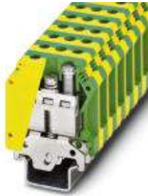
Ground modular terminal block, Connection method: Screw connection, Load current : 150 A, Cross section: 0.75 mm 2 - 50 mm 2 , AWG 18 - 2, Width: 15.2 mm, Color: green-yellow
