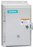
Non-reversing motor starter, Size 1, Three phase full voltage, Solid-state overload relay, OLRelay amp range 3-12a, 240V 50HZ / 277V 60HZ coil, Non-combination type, Enclosure type 12, Dust/drip proof for indoors, Extra-wide enclosure
