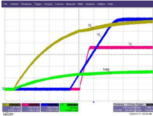
Fig. 7. Start up at 3A Load Ch 1 :V in , Ch 2 :V o , Ch 3 :V ss , Ch 4 :Enable
