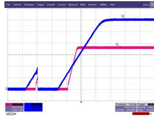
Fig. 12. Short (Hiccup) Recovery Ch 2 :V o , Ch 3 :V ss
