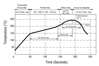
Peak Temperature: 245 °  $\pm 5$  °C max., 30 sec. max. Maximum Time Above 217 °C: 60~150 seconds
