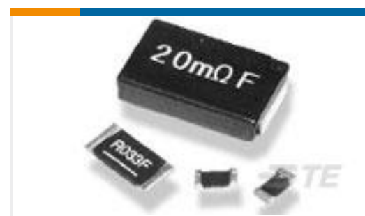
TE Part #3-1879378-3 TLR 2512 1.0W R004 1% 100PPM 2K RL
