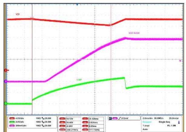
V_{DD} capacitor hold-up time = 8.9 ms V_{OUT} rise time = 9.1 ms CH2: VDD at 4 V/DIV CH3: COMP at 2V/DIV CH4: V_{OUT} at 4 V/DIV via differential probe Figure 9-13. V_{OUT} Soft Starting at 800 V_{IN} , 40 W
