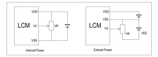
$V_{\text{DD-}}V_0$ : LCD Driving voltage VR: 10k~20k
