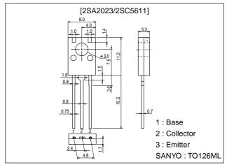
Note: The emitter and base are reversely assigned to those of our standard products encapsulated in the TO-126ML package.
