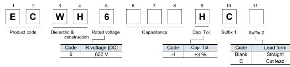
Rated voltage 630 V (Odd size taping)
