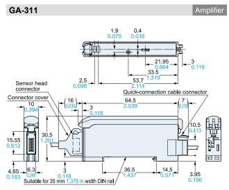
Note: The front view shows the sensor head connector and quick-connection cable connector attached. The top view is without the sensor head connector, quick-connection cable and the cover.
