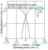
The graph on the left is plotted with the sensitivity adjusted so as to just detect a 10 × 10 × t 1 mm 0 394 × 0 394 × t 0 039 in iron sheet placed at a distance of 2.0 mm 0.079 in.
