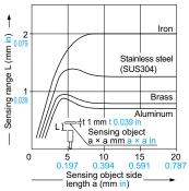
As the sensing object size becomes smaller than the standard size (iron sheet 10 × 10 × t 1 mm 0.394  $\times$  0.394  $\times$  t 0.039 in), the sensing range shortens as shown in the left figure.
