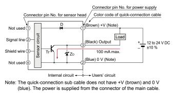
Symbols ... D : Reverse supply polarity protection diode ZD: Surge absorption zener diode Tr : NPN output transistor
