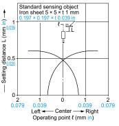
as to just detect a 5 × 5 × t 1 mm × 0.197 × t 0.039 in iron 0.197 sheet placed at a distance of 0.6 mm 0.024 in.
