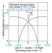
The graph on the left is plotted with the sensitivity adjusted so as to just detect a 5 × 5 × t 1 mm 0.197 × 0.197 × t 0.039 in iron sheet placed at a distance of 0.8 mm 0.031 in.
