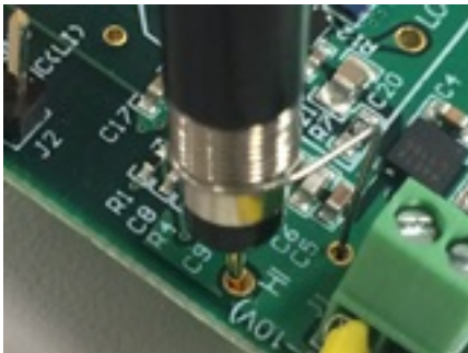
Figure 4. HI Test Point (TP8)
