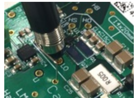
Figure 9. LO Test Point (TP11)
