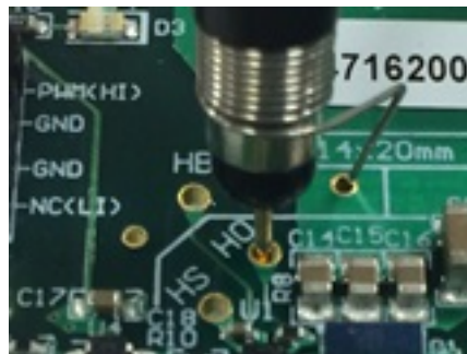
Figure 8. HO Test Point (TP3)
