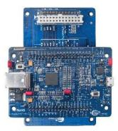
2. Plug the Aptina Image Sensor Board into the Aptina Image Sensor Interconnect Board (The Aptina Image sensor board is not part of this kit)
