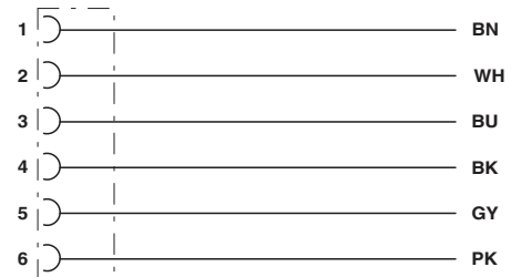
Contact assignment of M8 socket
