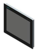
SIMATIC IFP1900 V2 Standard 5:4 19" multi-touch display (5:4) with 1280x1024 pixel resolution; built-in unit for 24 V DC; display port/DVI interface; including DP/USB cable 1.8 m; USB on the rear side; standard Siemens design
