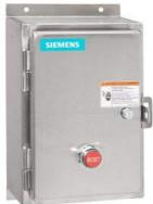
Non-reversing motor starter Size 2 Three phase full voltage Solid-state overload relay OLRelay amp range 13-52a 240VAC 50HZ / 277VAC 60HZ coil Combination type Water/dust tight non-corrosive
