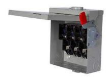
Siemens Low Voltage Circuit Protection General Duty Safety Switches. Type: ENCLOSED, SAFETY SWITCH Std: CSA V. Rating: 240V A. Rating: 200A Wattage: 4W No. Of Poles: 3P F. Rating: 60Hz Action: SINGLE THROW Material: STEEL Enclosure: TYPE 1. 2-3 point mounting holes. O. Cycles: 8000 O. Temperature: (-20F-120F) AMBIENT TEMPERATURE Environmental Conditions: INDOOR
