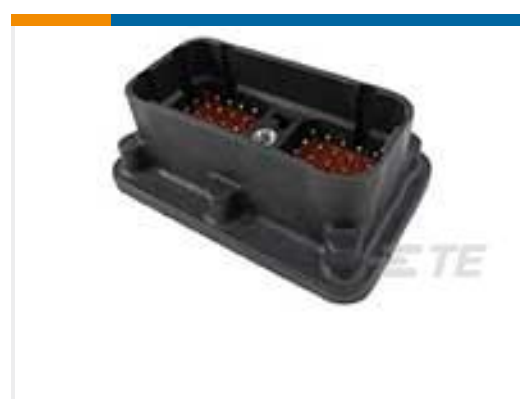
TE Part #DRC20-50P02 HDR, 50P, BLK, ST, AU/NI/CU, 02
