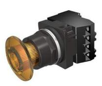
30mm BlackMax, Epoxy Coated Corrosion Resistant Complete Metal Unit Illuminated Twist-to-Release Full Voltage, 24V AC/DC LED Lamp Mushroom Head Cap Small 1.79" (45 mm) Plastic Cap, Amber 2 Position Maintained, Twist-to-Release with 1 N.O. - 1 N.C. Heavy Duty Contacts, A600/P600 UL Listed, CSA Certified NEMA 1,3,3R,4,4X,12,13 & Automotive Standards
