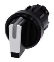
Selector switch, illuminable, 22 mm, round, plastic, white, selector switch, short, 3 switch positions I>O<II, momentary contact on the left, latching on the right, actuating angle 2x45°, 10:30h/12h/13:30h Z=50-unit packaging
