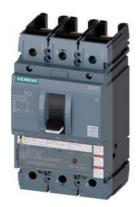
circuit breaker 3VA5 UL frame 250 breaking capacity class C 100kA @ 480V 3-pole, line protection TM210, FTFM, In=200A overload protection Ir=200A fixed short-circuit protection Ii=10 x In UL 489 SB (naval), 50° C without connection
