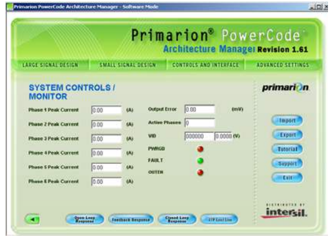
FIGURE 25. PRIMARION POWERCODE MONITOR WINDOW
