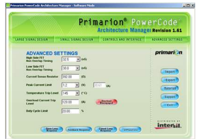
FIGURE 27. PRIMARION POWERCODE DUTY CYCLE LIMIT SELECTION
