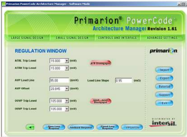
FIGURE 23. PRIMARION POWERCODE LOADLINE AND ATR SETTINGS
