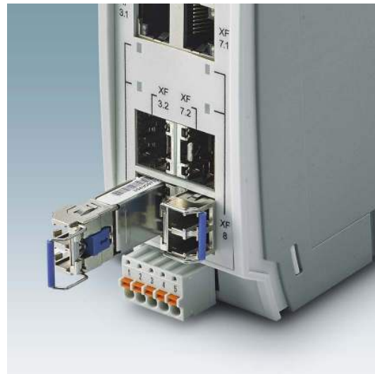
Figure 3-10 Inserting the SFP modules (example)
