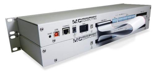
The TC-32 can connect to an Ethernet or USB port. Both the TC-32 and TC-32-EXP include 50-pin connectors that provide access to all DIO channels. Adding the TC-32-EXP expansion device doubles the channel count of the system.
